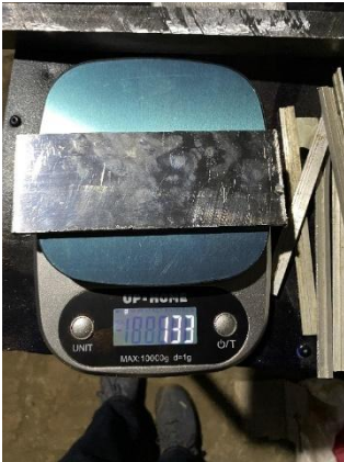
Penimbangan alumunium 95% 133 gram
