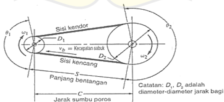
Gambar 2.3. Dasar-dasar geometri V-belt
