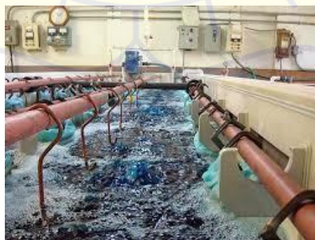
Gambar 2. 3 Proses Tembaga Plating [13]
