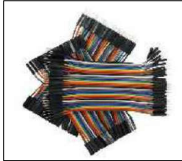
Gambar 2. 8 Kabel Jumper (Sulistyorini et al., 2022)
